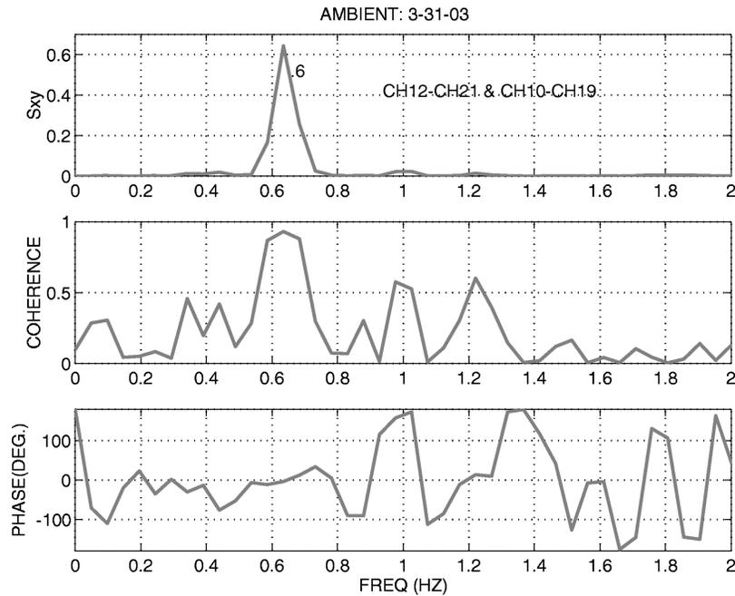
**Figure 8.** Cross spectrum, coherency, and phase angle plots of ambient acceleration response data obtained from differences of parallel channels, CH12–CH21 at the roof and CH10–CH19 at the 18<sup>th</sup> floor.
