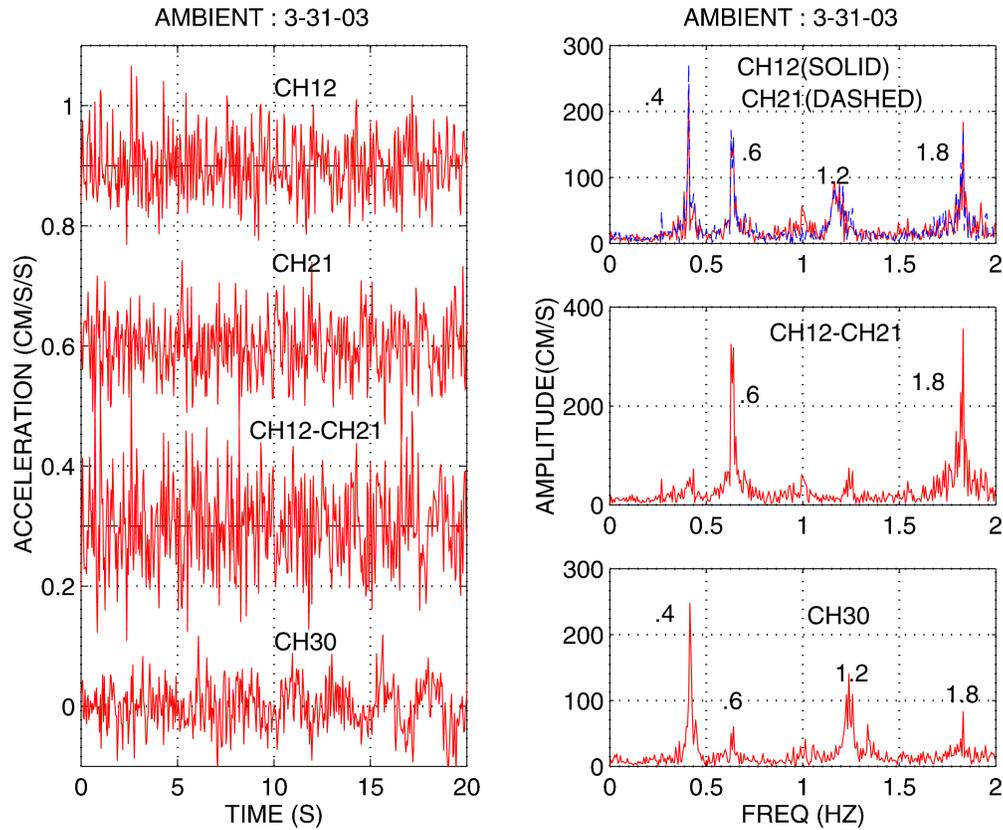
**Figure 6.** Twenty seconds of ambient acceleration response data obtained at the roof from parallel channels (CH12 and CH21), their difference (CH12–CH21), and from CH30, orthogonal to CH12 and CH21 (left) and corresponding amplitude spectra (right).
